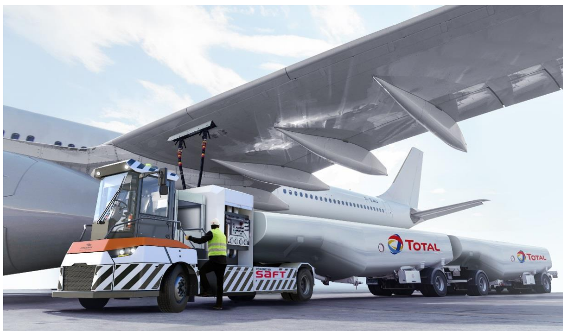
Electric Aircraft Refueller Transporter ART FULL ELEC®, equipped with two 30 tons fuel tanks (artist rendering – courtesy of Gaussin)
