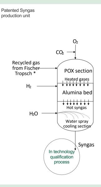
The Nordic Blue Crude POX-rWGS reactor design for producing e-fuel from CO2 and hydrogen represents a breakthrough in simplicity and reliability.
