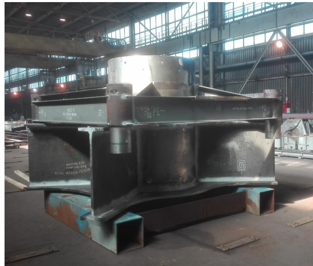
Well Bay Insert: finished fabricated 28.03 at EPG Poland, ready for painting
